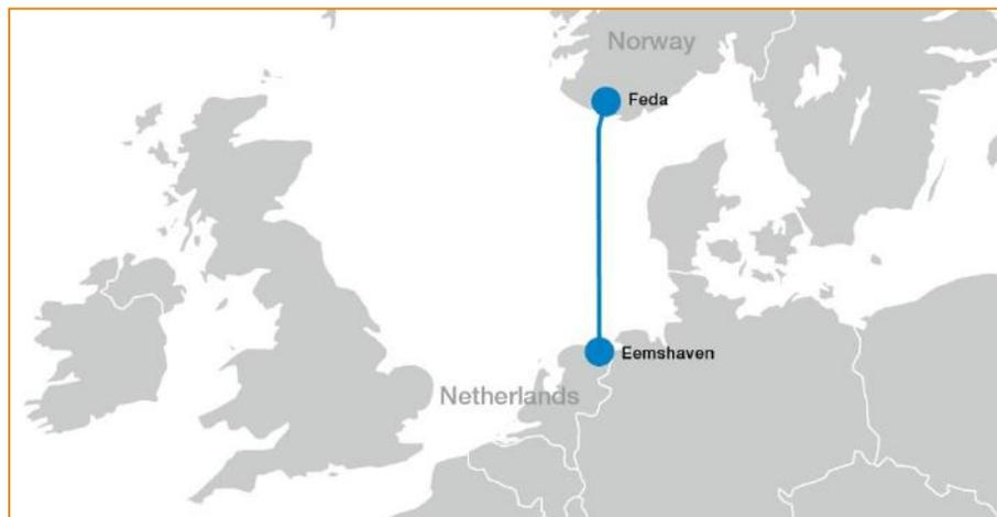
Image 2: The NorNed HVDC cable in Europe, connecting Feda, Norway to Eemshaven, Netherlands<sup>10</sup>
