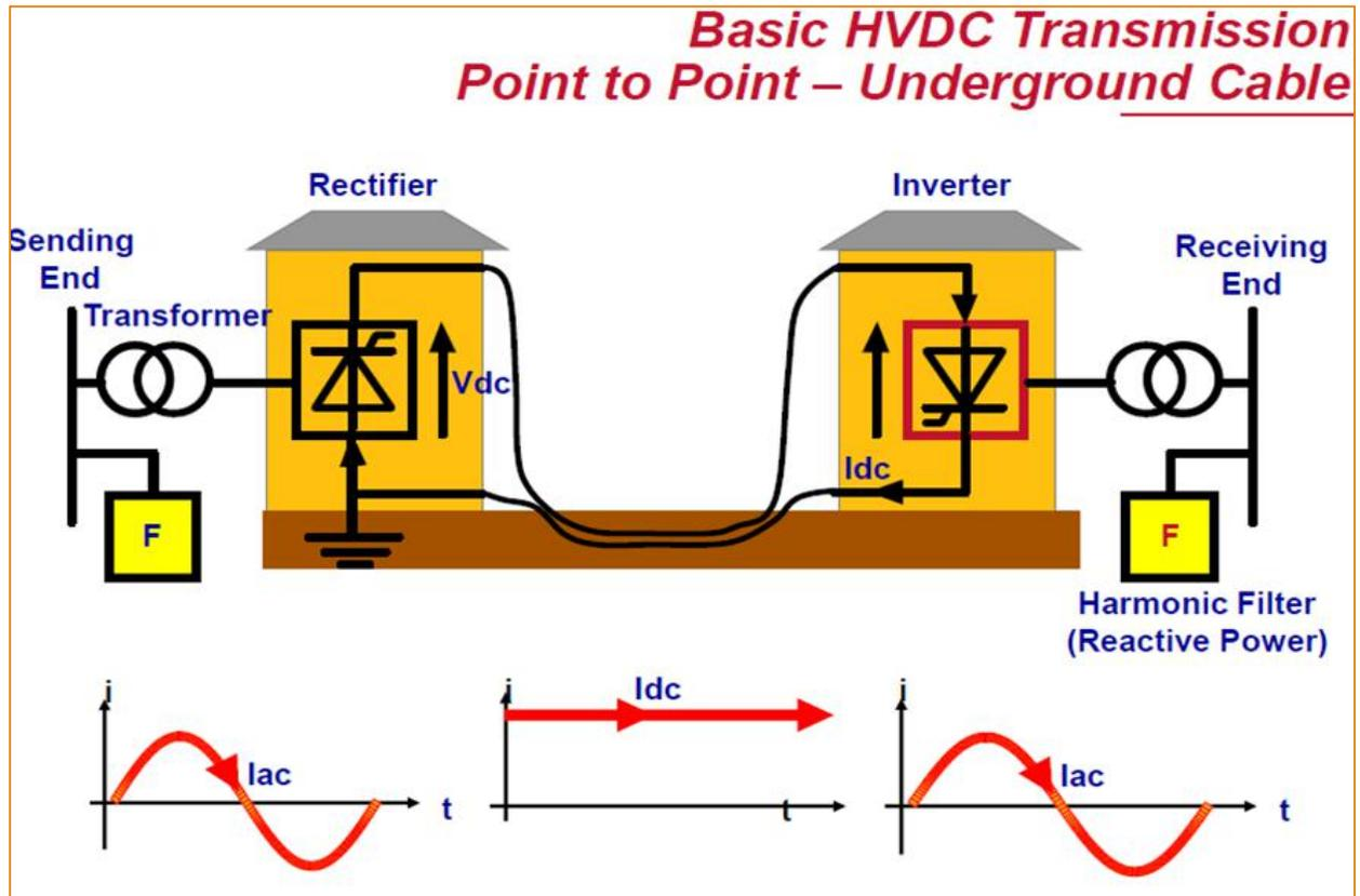
Here, choice of DC voltage is set by the cable to the highest possible voltage to minimize losses and cost.
