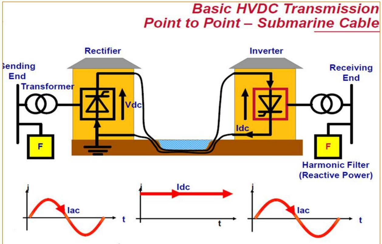
Here, choice of DC voltage is set by the cable to the highest possible voltage to minimize losses and cost.
